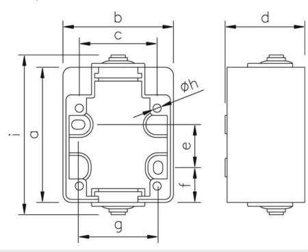
for sockets acc. to DIN 49440 with flange 50x50mm (exception: 1013-0b and 1025-0r)
